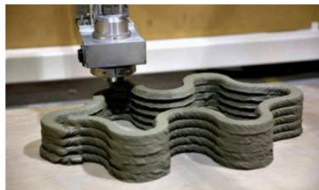
Going hi-tech: 3D concrete printing replaces traditional masonry and sequential manual labour with a computer-controlled system.
